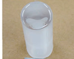
Fig.5 A resin model of the inner shape of a hose
